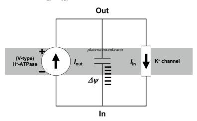
Requirement for steady state  $\Delta \psi$ :  $I_{in} = I_{out}$
