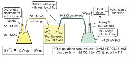
Using this technique, we have recently measured LJPs in diluted solutions of LiCl and NaCl (with and without 4 mM  $CaCl_{2}$ ) and found them to agree within the experimental error (0.1 to 0.2 mV)to those LJPs calculated with the Henderson equation (using ion activities. rather than ion concentrations, and using the Windows version of the liquid junction potential program JPCalc;
